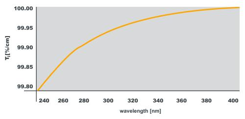
HPFS® KrF Grade is certified to meet  $T_i \ge 99.8\%/\text{cm}$  @248 nm when measured through a polished, uncoated sample.
